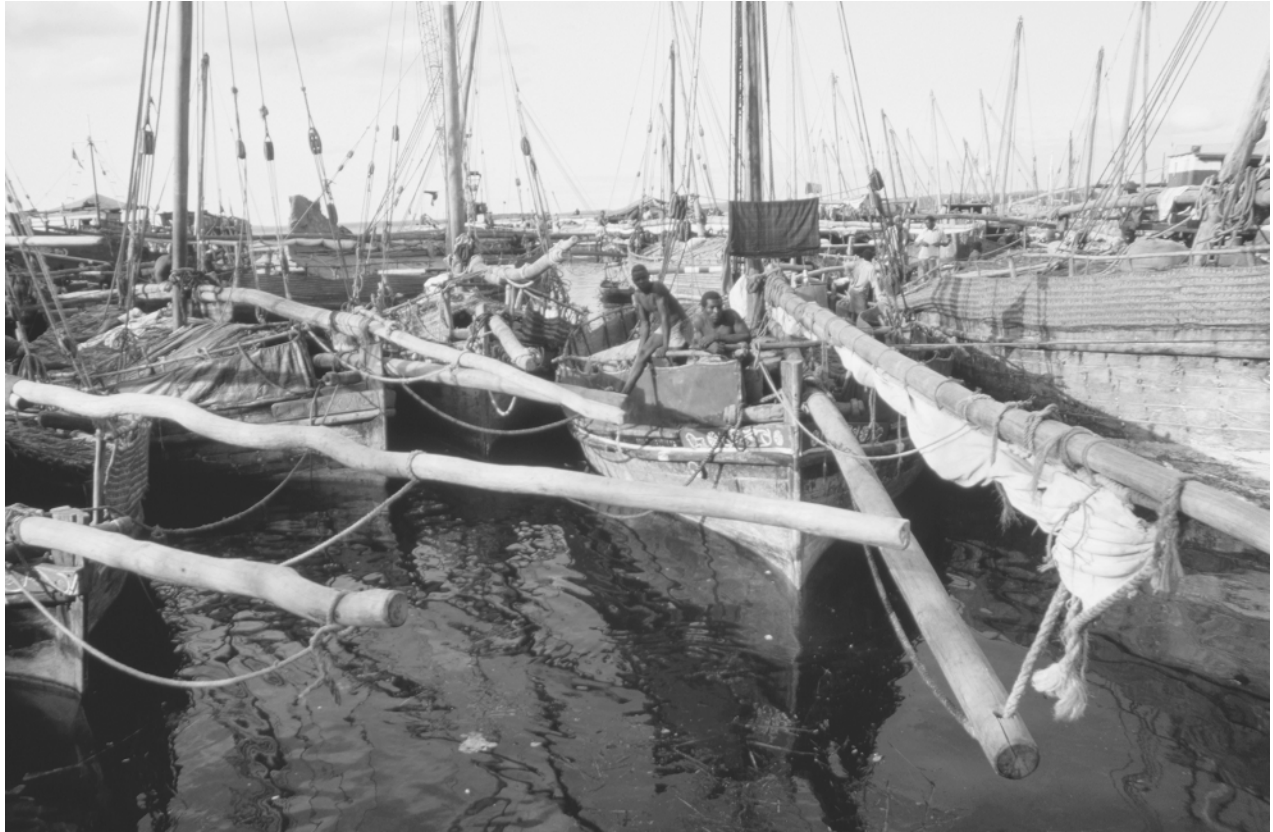
Arab dhows in Zanzibar Harbor. These wooden sailing boats transport cargo between the mainland and the Indian Ocean islands. They are specially designed for the monsoon winds in the Indian Ocean. They are quick, have no keel or motor, and can be easily stranded on the beach during low tide. © BOJAN BRECEL/CORBIS
