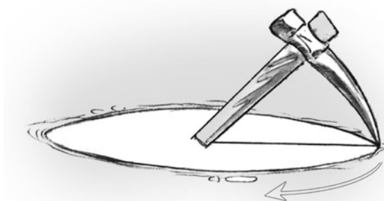
Fig. 4.13 Using a pick axe to determine the well radius
