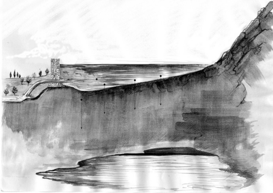
Fig. 7.12 Artificial recharge dam
