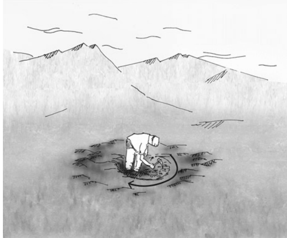
Fig. 4.16 A well is dug in a clockwise spiral way
