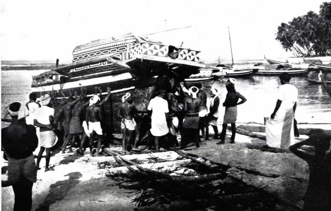
Sliding an odom onto palm-wood runners, ready for hauling up the beach
